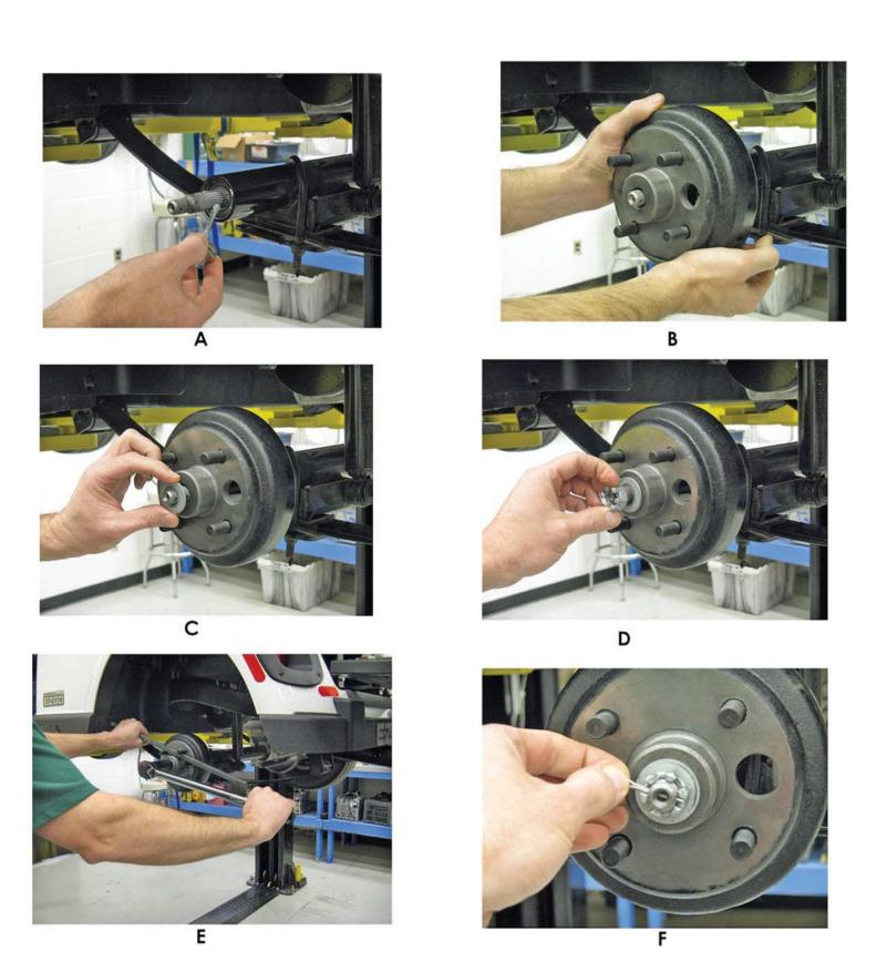
Install Anti-Seize on the axle shaft (A). Slide drum on shaft (B). Install flat washer (C). Install nut (D). Torque nut to 70 foot pounds (E). Tighten until cotter pin can be installed (F). Never back nut off for pin installation! Wear appropriate eye protection!
